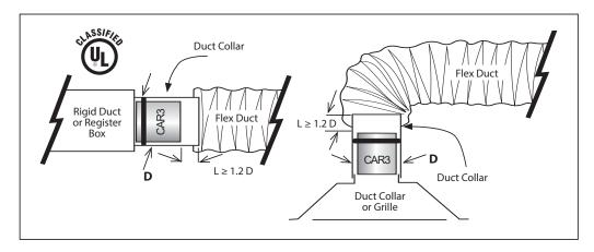
The CAR3 should be installed in accordance with all applicable building and mechanical codes. If installed in a metal duct or duct collar with a flexible duct connector (listed to UL 2043), the CAR3 must be inserted at least 1.2 times the duct diameter from the flexible duct and/or duct connector.
